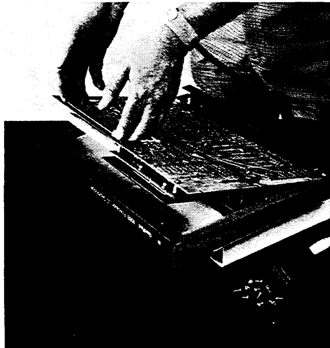
Figure 5-8. Removal of the main board from the 1689 Digibridge. The ribbon cable must be disconnected first. Prior removal of the display board also is highly recommended. Because the board is partially enclosed by the main chassis, unusual care may be needed in removal. These motions are suggested: slide toward the rear, tilt as shown, and gently lift free.
